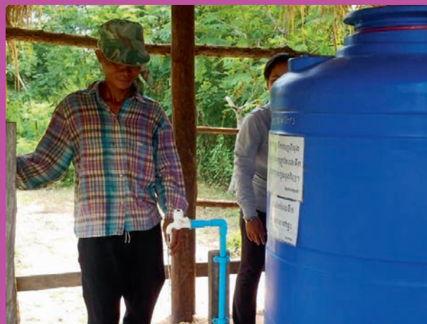
A bio-sand water filter system with instructions in Khmer language
