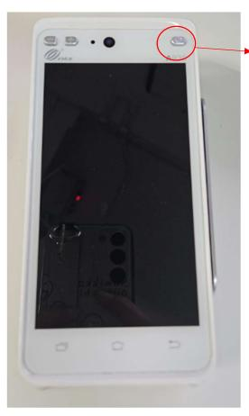
Press and hold power button for 5 secs. Until you hear a beep sound. The screen will light up as below
