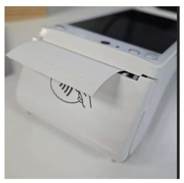
After change, please ensure that there's a bit of paper sticking out of the machine before closing the lid.
