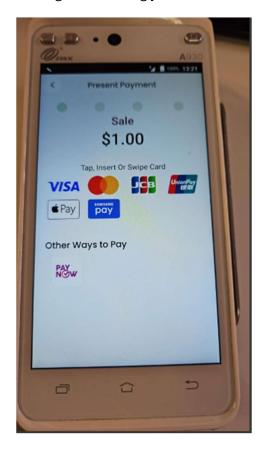
Tap or insert credit card into the terminal. When successful, the below screen will light up. The merchant receipt will also start to be printed.
